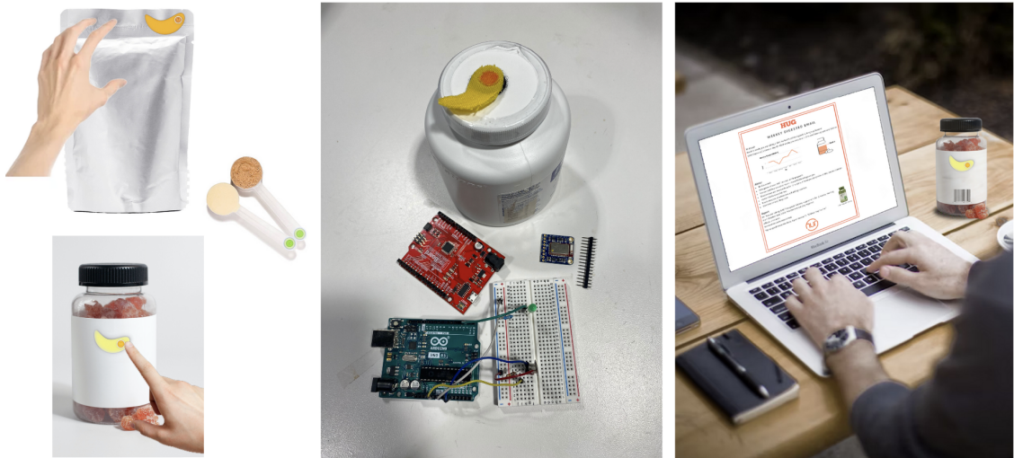
Fig. 2. (Left) HUG Smart Sticker on three different medication packagings; (Middle) HUG Smart Sticker's hardware module; (Right) HUG Smart Sticker's software module.
